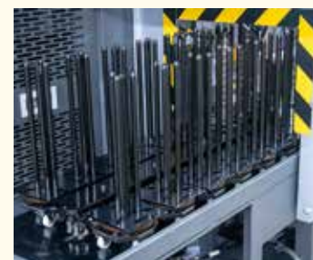
● Station Stocker Flexible Multi-layer stocker to accommodate different part diameter sizes.
