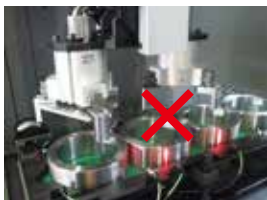
Interference with the loader on one side
