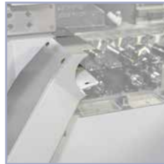
Work catcher The workpiece is discharged from back spindle into the chute of the catcher, and carried out to the work conveyor. ●3290-Y3070
