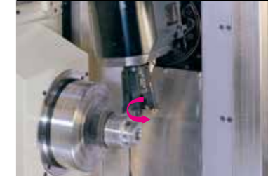
Multi turning holder to index in 4 positions
