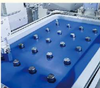
● Tray Changer Workpieces can be stored in individual trays.
