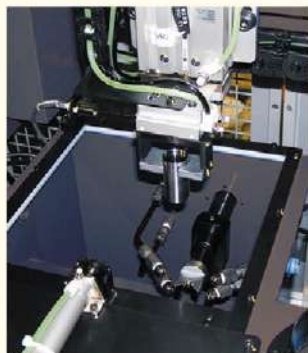
● Cleaning Unit Without operator intervention, cleaning is performed automatically.
