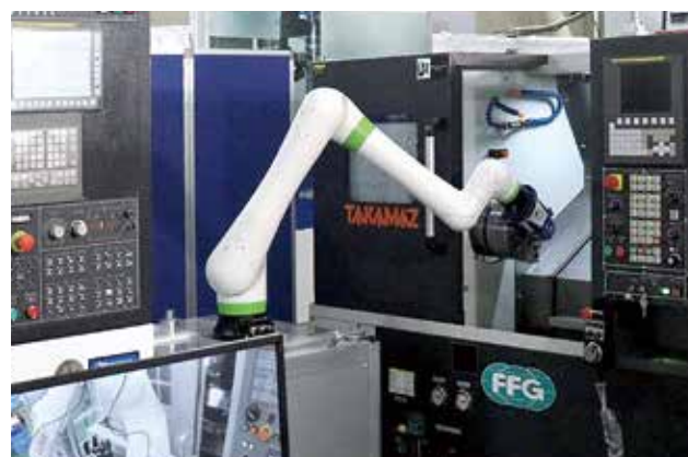
Example of use : HV-32A (FEELER) + CRX (FANUC, robot) + T-6i (LEADWELL)
